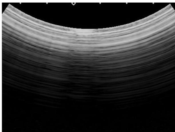
Fig. 2. Suspected delamination of the acoustic stack, indicated by disruption of the reverberation pattern.
