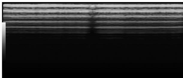
Fig. 3. Reverberation pattern revealing atypical central dropout where the FirstCall result indicated no fault. The dropout is atypical as the axial shadow does not extend to the top of the image.
