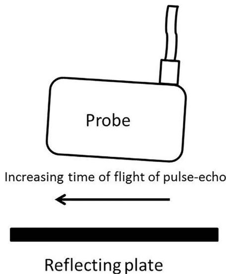
Fig. 1. Probe position for time-of-flight measurement to check array sequencing; time-of-flight should increase linearly from right to left of the diagram.
