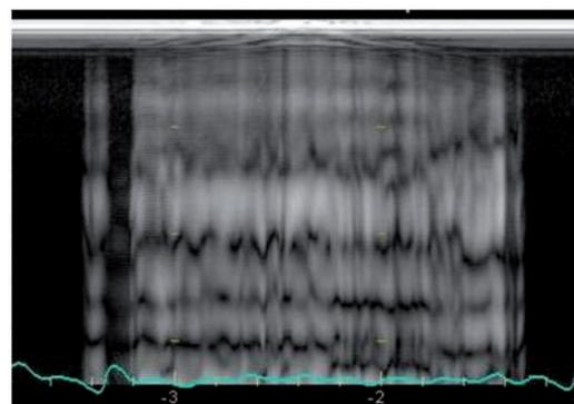
**Figure 2.** M-mode paperclip test showing dropout towards one end of the array (dark axial band towards the left of the image).
