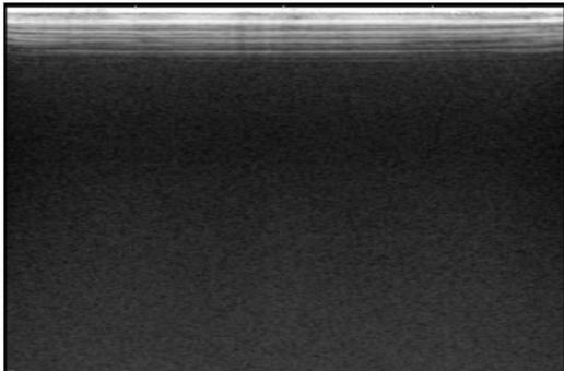
**Figure 3.** Minor lens wear shown by a change in depth of reverberations at the ends of the probe, and minor non-uniformity shown by faint axial streaking in the reverberation pattern.
