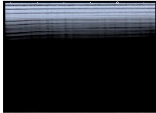
**Figure 4.** Significant lens non-uniformity (>5% variation in reverberation depth).
