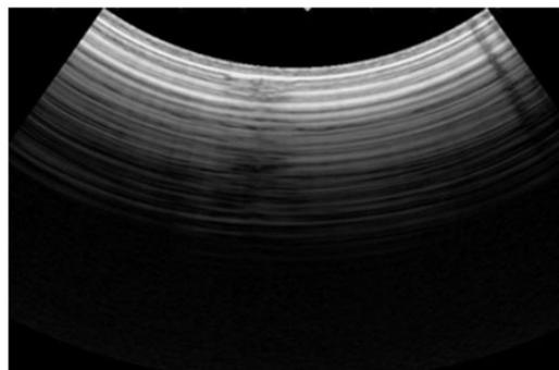
**Figure 1.** Drop out (axial streak on the right) and delamination (disrupted reverberation pattern to left of centre) on a curvilinear array.
